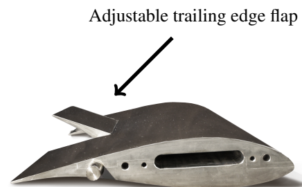
FIGURE 2. Test aerofoil with trailing edge flap
