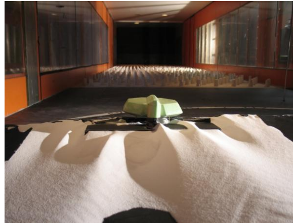
Aerodynamic design of the Belgium polar station (VKI)
